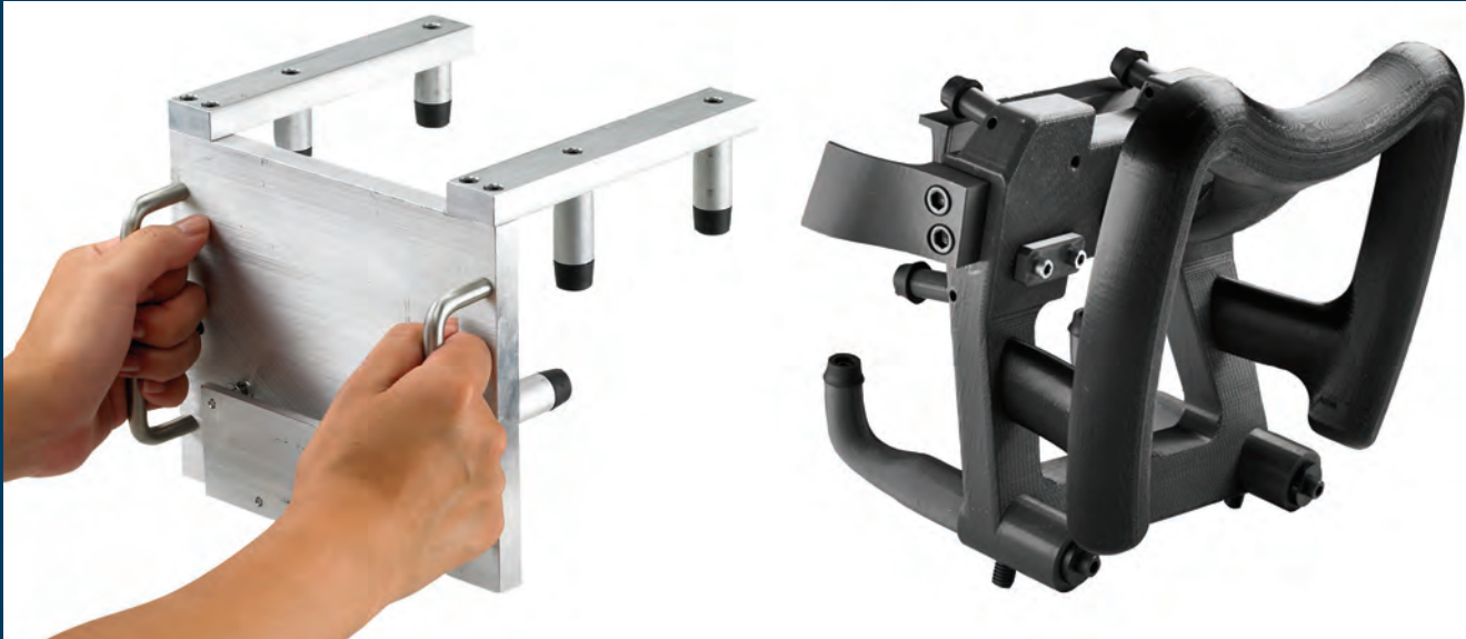
BMW used Fused Deposition Modeling to design lighter fixtures with design complexities.
