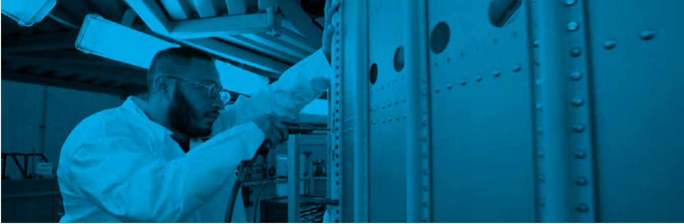
A production floor worker uses a jig to aid with drilling.
