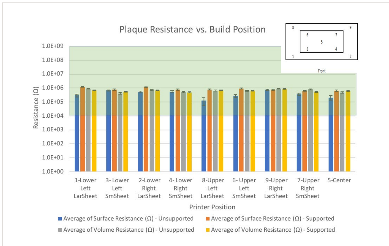
Figure 6. Plaque build position vs. part resistance.
