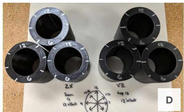
Figure 2. Examples of test parts for ESD suite. A) plate, 45 degrees. B) plate, edge (ZX). C) thin (0.05 wall) cylinder. D) thick (0.20 wall) cylinder.
