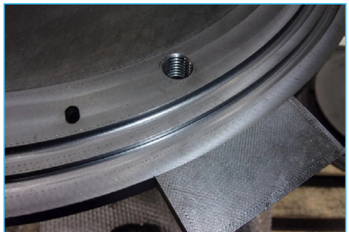
A view of the 3D printed center and base sections machined for threaded inserts, O-ring grooves, locating holes, and flat sealing faces.
