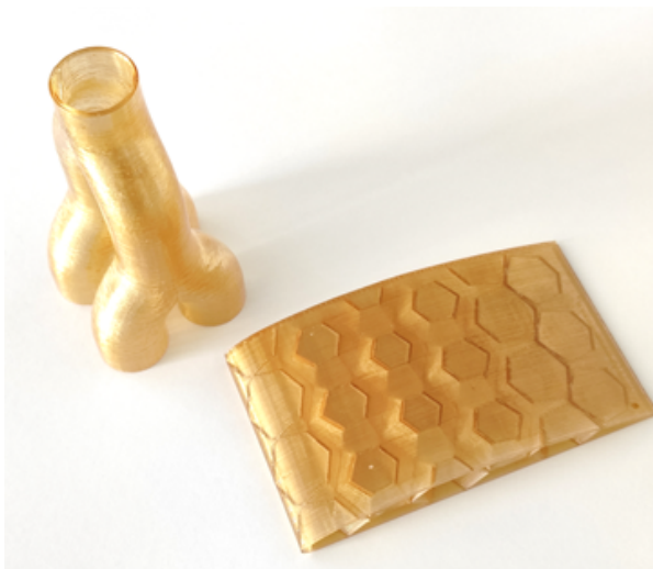
3D printed aerospace parts that have been vapor fused.
